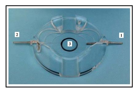
Perfusion solution enters from one side [1] via a stainless steel tube and exits through a well [2] in which a movable tube attached to a pump/ suction line adjusts the fluid level. Solutions can be prewarmed before entering the chamber with our Mini Heating Module MH01. The profile slopes in towards the central coverslip base [3] so that the perfusion solution forms a pool around the preparation whilst being refreshed by virtue of the inlet and exit ports.
