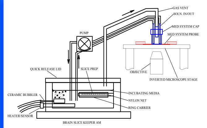
Pipes and tubes should be as short as possible and arranged to be well thermally insulated to minimise the temperature drop from the incubating area to the recoding area. The PTC03 temperature controller is electrically quiet and should not produce any interference in recordings. Peristaltic pumps may need to be grounded and shielded and kept at a distance from the recording area.
