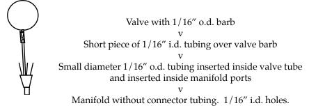
Cutting the tubing at an angle will make insertion easier. Cutting the tubing square, however, will minimize dead volume when inserted as far as possible into the manifold – being careful not block at the point of convergence.
