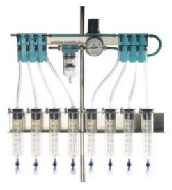
The package can be added to any new or existing perfusion rig - from AutoMate Scientific, any third-party manufacturer, or even homemade. Connect to house air, tank, or compressor (30 to 100 psi). Precision regulator delivers zero to 10 psi to pressurized syringe reservoirs.
