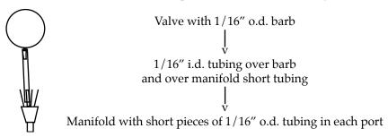
... or, for even **less dead volume**, use a short piece of 1/16'' <u>i.d.</u> tubing over the valve barb, and piece of smaller 1/16'' <u>o.d.</u> tubing inserted inside the valve tubing and manifold ports (you may need to supply extra small tubing for this option):
