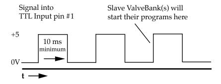
Note: TTL Input #1 can still be used on slave ValveBanks after their start signal.
