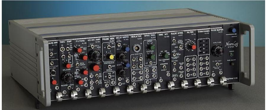
The **NL900D Case & Power Supply** unit allows up to thirteen modules to be installed. This means that a single NeuroLog System can be used to amplify several different parameters, such as extracellular spikes, intracellular potentials or even blood pressure, as well as produce outgoing trigger pulses to other pieces of equipment or electrically stimulate a preparation.
