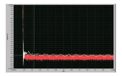
Same as graph above, using patented vibration-cancellation technology. The undesirable rapid switching of the HEKA amp output (red) due to rapid recoil-driven structural oscillations of the theta glass is eliminated.
