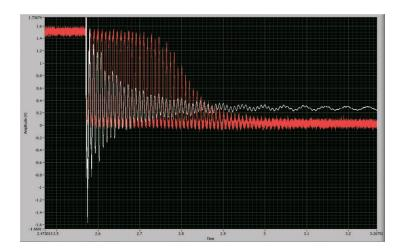
Rapid theta-glass transitions cause ringing of the mechanical structure. Zoomed-in view at target position. White: vibrometer real-time position output. Red: HEKA amp current. Correlation between physical position and HEKA amp output is evident. The vibration of the theta-glass pipette assembly causes repetitive switching of the patch-clamp signal.
