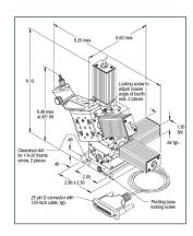
The closed loop connection ensures 0.2 µm and 0.1 µm resolution, respectively.
