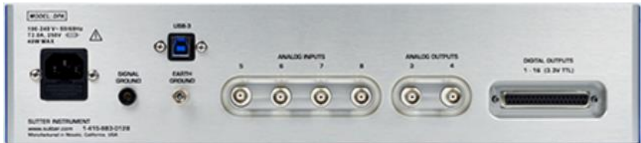
Figure 2-1. Rear of dPatch Cabinet
